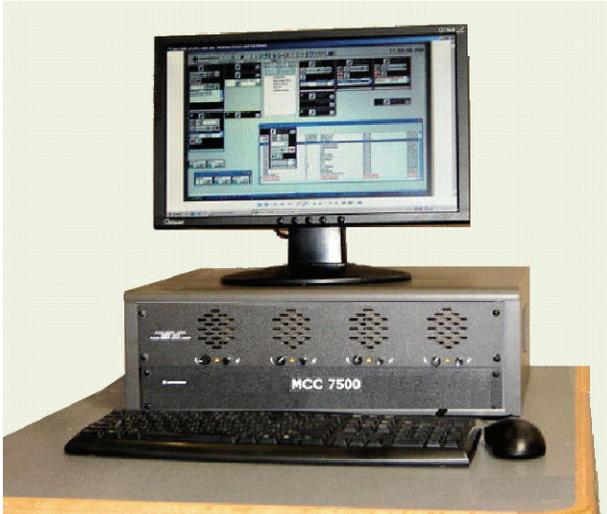
Four ISP's without microphone mount in 3RU Desk Top Cabinet. CIE and accessory mounting tray below speaker panel. LCD Stand on top of Cabinet.
