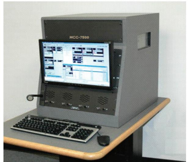
Four ISP's with microphone mount. LCD mounting kit above. CIE and accessory panel located in top section. Shown in special Prison Desk Top Cabinet.
