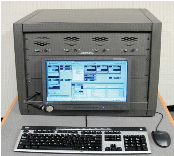
Four ISP's with microphone in Upper Turret with LCD mounting kit below. CIE and accessory panel behind speaker panel.
